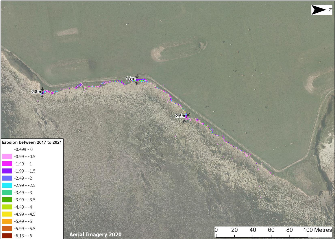
Figure 7 – Lidar comparison plot between 2017 and 2021 for Area D and F.
