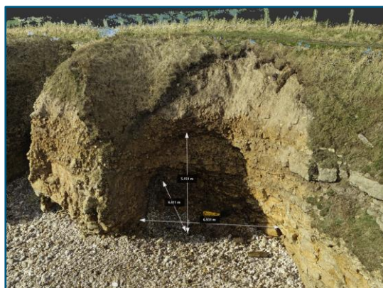
Cave 5 (Area F) – Approximately 7m wide, 5m high and 4.5m deep (Left) Image from drone survey (Right) Annotated RGB point cloud
