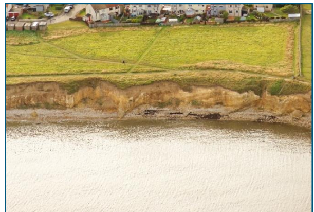
Area C – Magnesian limestone rising in elevation, resulting in steeper, harder cliffs. (Left) Image from site walkover (Right) Oblique Aerial Image from Cell 1 monitoring programme.
