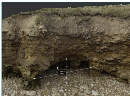
Cave 3 (Area C) – Approximately 8m wide, 3m high and 4m deep (Left) Image from drone survey (Right) Annotated RGB point cloud
