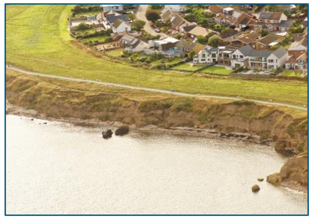
Area B – Thick glacial till deposits mantled on thin limestone shelf. (Left) Image from site walkover (Right) Oblique Aerial Image from Cell 1 monitoring programme
