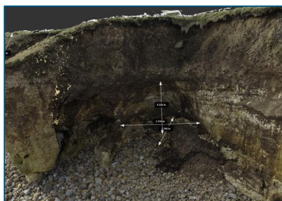
Cave 2 (Area C) – Approximately 4m wide, 4m high and 2m deep (Left) Image from drone survey (Right) Annotated RGB point cloud
